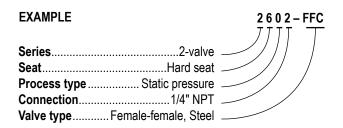
To meet all of your specific application requirements, the following **additional options** are available for these manifold valves. To order all or any of these options, simply add them to the part number as shown in the diagram below.
