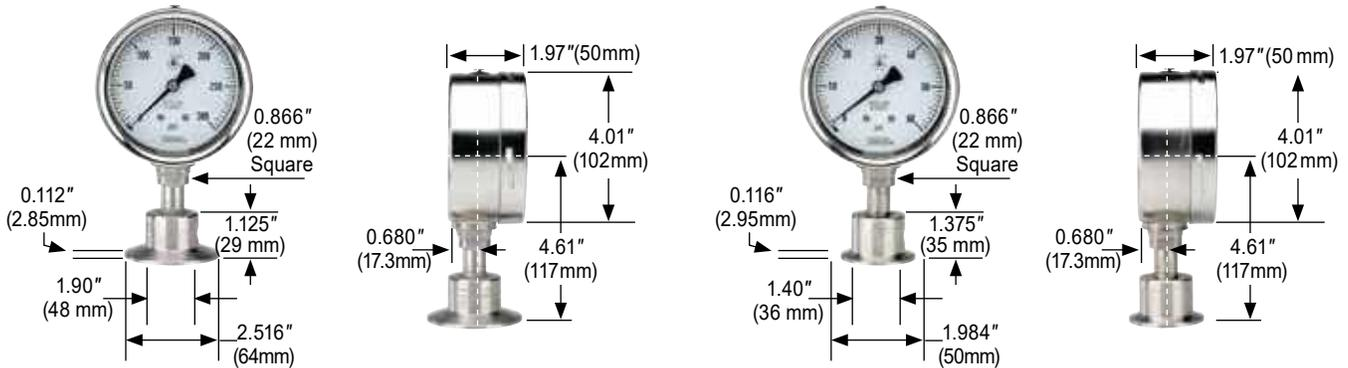
**2-1/2" Gauge with 2" ASME-BPE Sanitary Clamp Connection 2-1/2" Gauge with 1-1/2" ASME-BPE Sanitary Clamp Connection**
