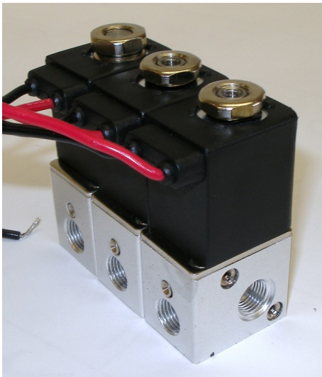
Figure 1: Parts of a 2V1 and 3V1 assembly. When connected, air flows through the inlets/default outlets, which are the horizontally oriented ports in this picture. The vertically oriented ports in the 3V1 valves are connected to the exhaust, which is above the black solenoid coils.
