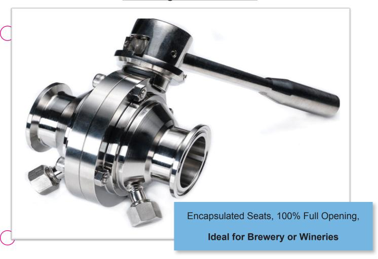
Sanitary Solutions is your source for a full port, cavity filled, T304 clamp connection dual purge port ball valve. Our dual purge port ball valve is constructed with a full port positioned inside the valve body between two polished flanges and two Teflon® valve seats. Do you see the two purge ports located at the bottom of the valve for full drain ability, taking samples, and CIP/SIP applications?
