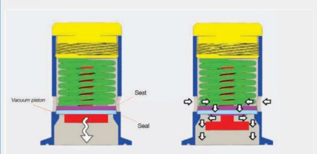
Normally closed, but when there is a vacuum in the tank, the vacuum piston opens automatically, drawing air into the tank. Thus, keeping pressure balance. inside and outside the tank
