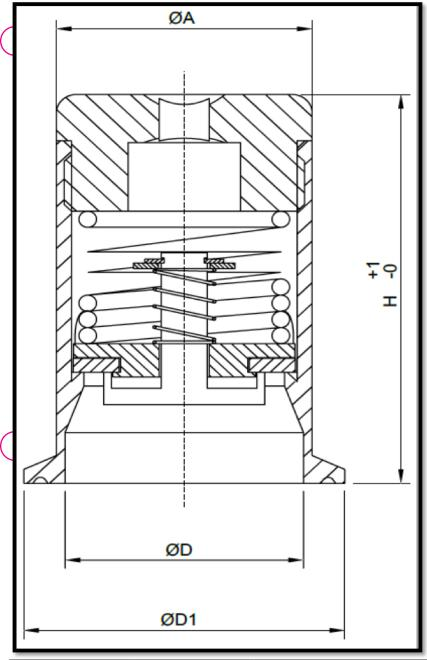
Tank Pressure-Vacuum Relief Valve Part Number:
