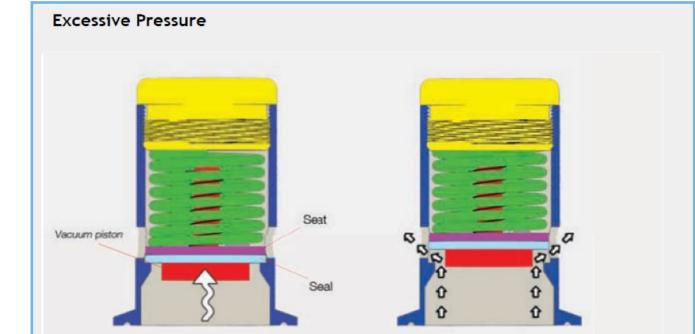
Normally closed, but when the tank pressure exceeds the rated pressure, the valve automatically opens to vent air out.
