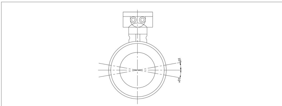
At flow meter upstream, there should be straight pipe no less than  $5D$  and no less than  $2D$  at flow meter downstream. ( $D$  is the inner diameter of the flow meter)
