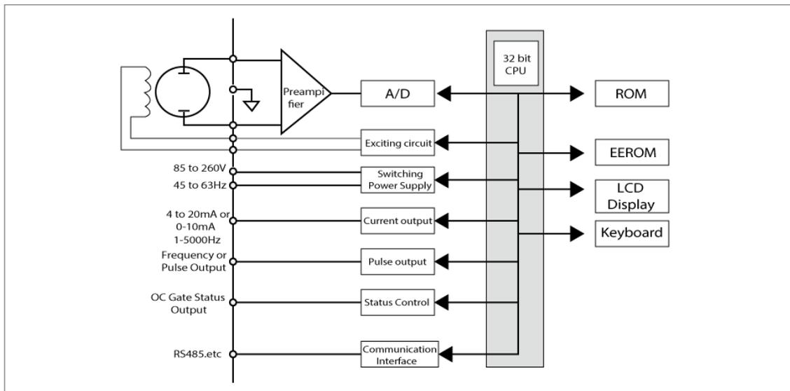
The converter can supply the exciting current to the coil in the sensor of electromagnetic flow meter; the head amplifier amplifies the electromotive force from the sensor and converts it into standard signals of current or frequency so that the signals can be used for displaying, controlling, and processing.
