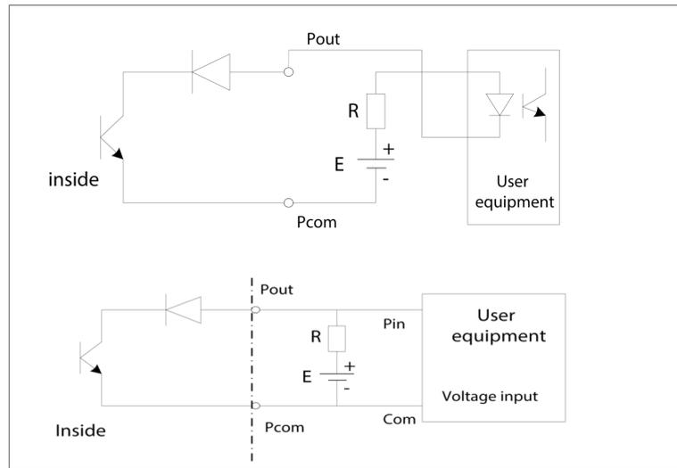
Commonly, the user's photoelectric coupling current is about 10 mA, so  $E/R=10$  mA, where  $E=5$  to 24V.
