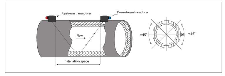
The V method is a standard installation method and convenient to use for precise measurement of flow. While installing the two transducers, they are horizontally aligned. The transducers center lines are parallel with the pipe axis line. They are suitable for pipe diameter range 1/2" to 16" (DN15 mm-DN400 mm).
