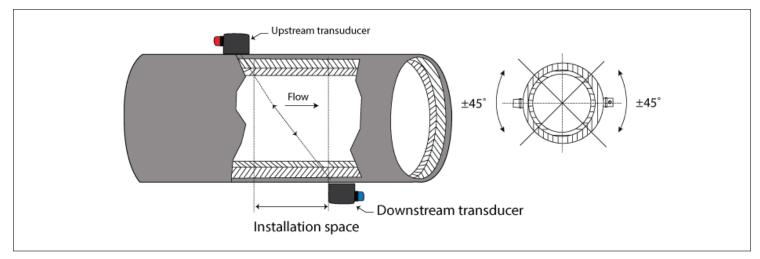
When the pipe diameter is wide, there are suspended matters in the fluid, or the scaling is too thick, it can interfere with the normal functioning of the flow meter, this weakens the signal in a V method installation. If this happens, the Z method of installation is used. It is also called the single sound path as it can directly transfer the pulse without any reflection required, which is required in V method and therefore has less signal attenuation.
