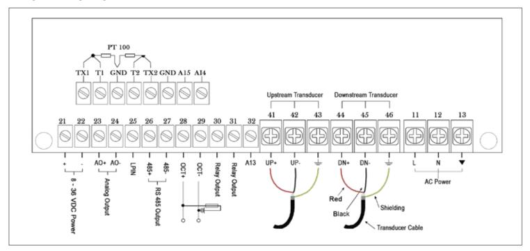
• Signal Wiring Diagram of 1200A-100M
