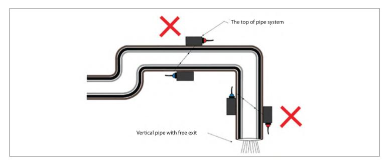
• For an open pipe or half full pipe, transducers should be installed at the bottom of the U pipe.
