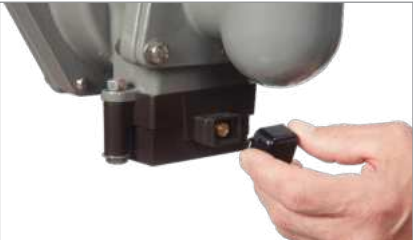
1. Remove the dust cover from the sensor.
