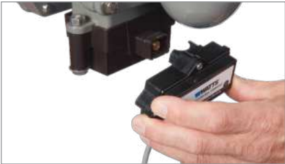
2. Press the activation module onto the sensor.
