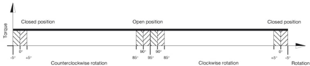
With reference to the above diagram it can be noted that the torque of a double acting actuator remains constant through-out the complete action. The user can decide on which model to choose according to his/her own specific requirements, using the following guidelines:
