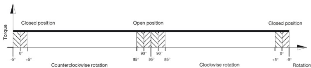
With reference to the above diagram it can be noted that the torque of a double acting actuator remains constant through-out the complete action. The user can decide on which model to choose according to his/her own specific requirements, using the following guidelines:
