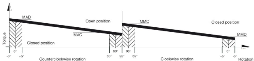
With reference to the above diagram the torque of a spring return actuator is not constant but decreasing. This is due to the action of the springs that when compressed during air actuation counteract the piston movement and accumulate energy which will be available in a decreasing way during the rotation inversion.
